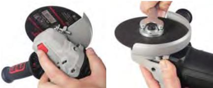
► After fitting the abrasive tool, check that the abrasive tool is fitted correctly and can turn freely before switching on the power tool. Make sure that the abrasive tool does not brush against the protective guard or other parts.
