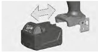
**1** Remove the battery pack before starting any work on the machine.
